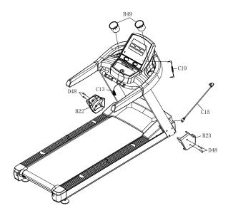
**ATTENTION:** Must confirm complete assembly as the required above and lock all bolts. Do the following operations after checking everything is OK. Before you use the treadmill, please read the instructions carefully.
