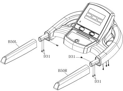
**Step 4:** Connect the cables (C16) of console and cable (C18) of right upright then tighten console with Left /Right upright (A3L/R), then secure Right/ Left upright (A3L/R) and Cross bar (A4A) with Round hex bolt M10\*20 (D105) and Flat Washer M10 (D21). Secure all screws on uprights. Then, connecting the Pulse upper line (C39) and Pulse bottom line (C40).
