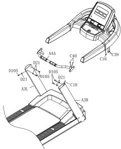
**Step 5:** Use Cross self-tapping bolt ST4.2\*19 (D48) to secure Left/ Right motor side cover (B22/23) to Left/ Right upright (A3L/R).
